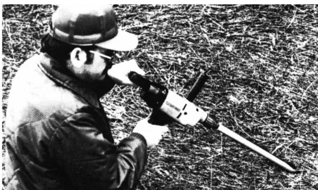
Figure 1. Forage probe mounted on an electric drill.
