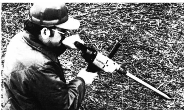
Figure 1. Forage probe mounted on an electric drill.
